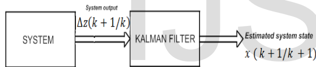
Fig.1 Kalman Filtering a System Output to Optimally Estimate the System State.[2]
